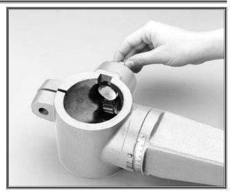
Figure 9. Insert the pinion gear from the inside.
